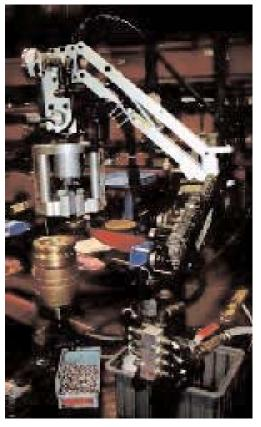
This fuel nozzle test rig uses pneumatic cylinders to actuate nozzles to failure — typically more than 1 million cycles. The rapid motion of pneumatics, plus the cushioning effects of compressed air, provide a motion dynamics that would be expensive and complicated to achieve using other technologies.
