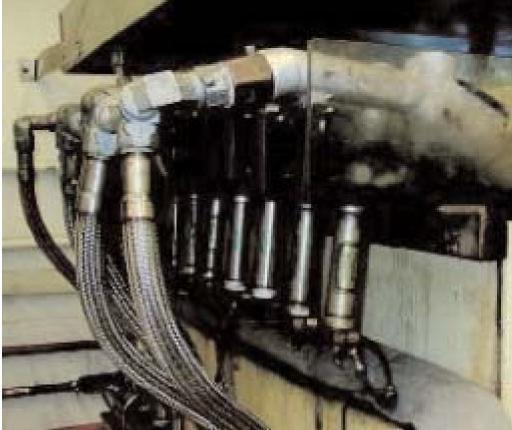
This automated test rig checks torque required to thread mating parts together. Because torque is limited by pressure supplied to a rotary actuator, the rig errs on the side of caution - even though some good parts may be rejected, it can pass only good parts.
