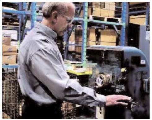
This press features features a pneumatic control that requires the operator keep both hands on pushbuttons — safe and out of harm's way. Implementing this and safety practices has helped contribute to more than a 90% reduction in workplace injuries.
